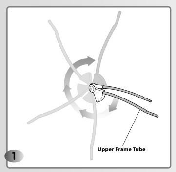
• Rotate the upper frame tube until it "snaps" into an upright position, as shown.
